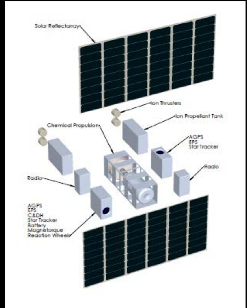
\* Alternate 6U flight test article concept derived from NASA CubeQuest Challenge Team Alpha CubeSat design
